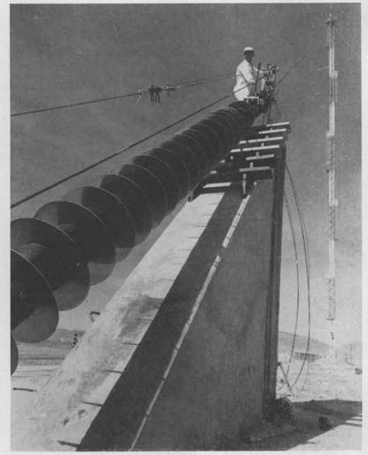
SHOCK ABSORBERS on 300-foot drop tower in Area III check recoil when cart descends cable. The tower is used to test the effects of shock on a variety of strategic materials.
